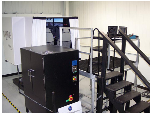
Fig. 5 WVU 6-DoF flight simulator system.
